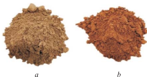
Fig. 1. Color of the clay sample before calcination ( a ) and after calcination ( b )
