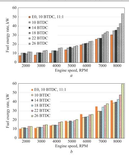
**Fig. 2.** Fuel energy rate on varying ignition timing and speed engine (*a*) and fuel exergy rate on ignition timing and speed engine variations (*b*)
