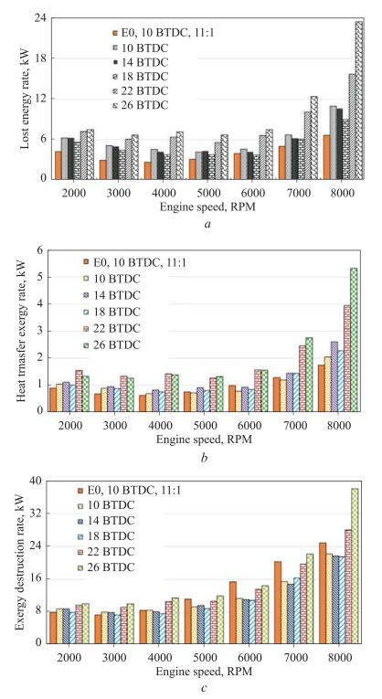
**Fig. 6.** Loss of energy rate (*a*), heat transfer exergy rate (*b*) and exergy destruction rate (*c*) on ignition timing and speed engine variations
