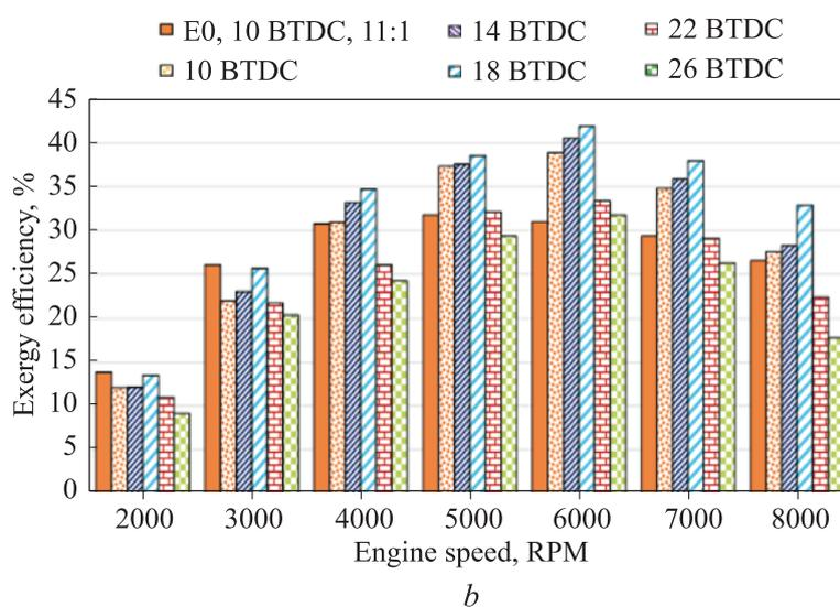
**Fig. 7 (end).** Exergy efficiency rate (*b*) on ignition timing and speed engine variations
